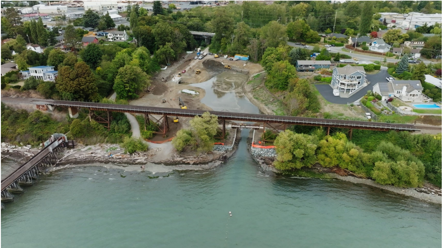
Aerial photo showing an overview taken immediately after inlet opening, and initial flooding of the site with saltwater from Bellingham Bay. (Photo Credit: BTV – City of Bellingham)
