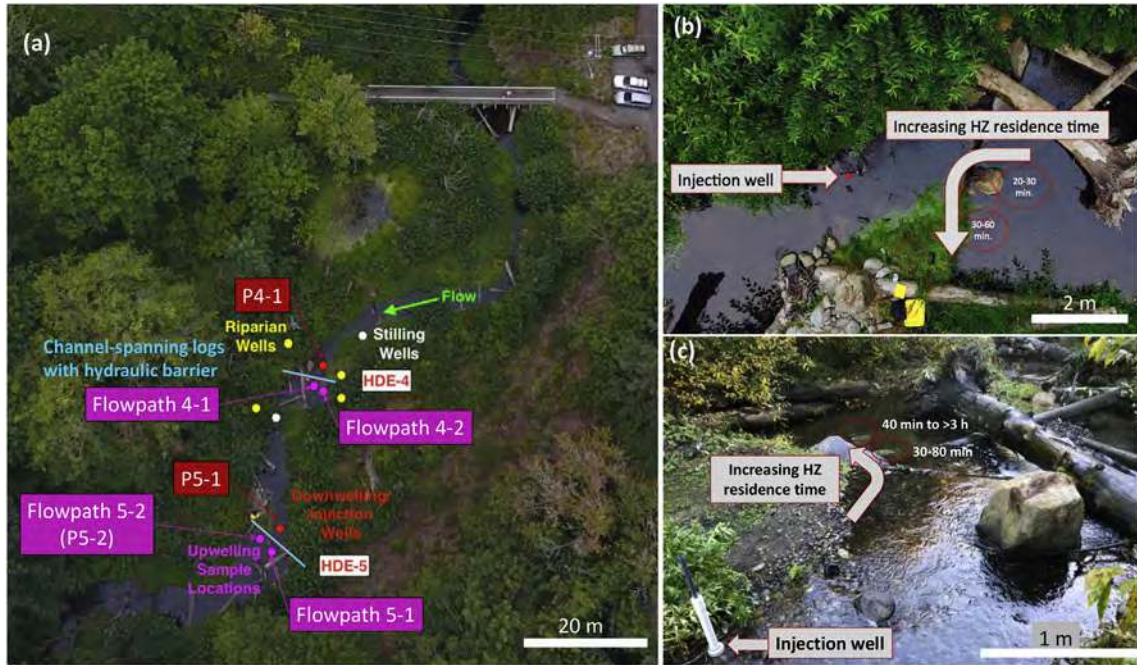
Fig. 1. (a) Map of study site within Kingfisher Reach on the South Fork of Thornton Creek showing hyporheic design elements (HDEs) and downwelling/upwelling sampling sites, and photographs of (b) HDE-5 and (c) HDE-4, showing locations of dye injection and upwelling, and approximate residence time distributions.
