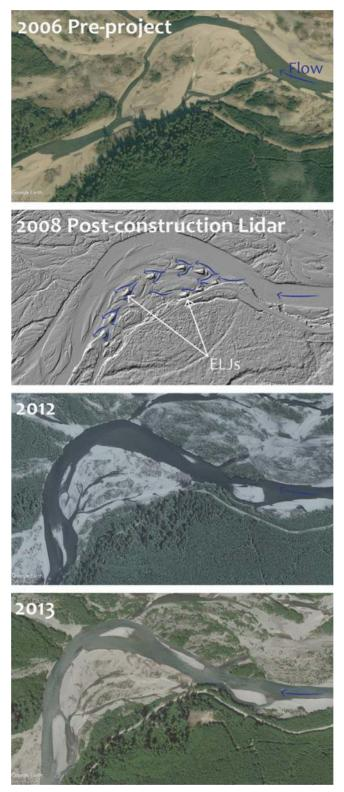
Fig. 4 Development of anabranching channel morphology using ELJs on the Upper Quinault River, Jefferson County, WA.
