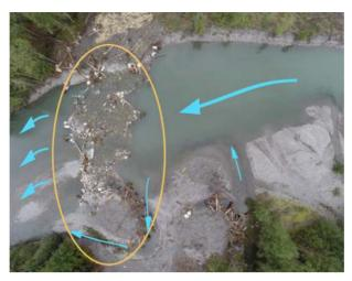
Fig. 7 Channel-spanning ELJs in Upper South Fork Nooksack river, Skagit County, WA.
