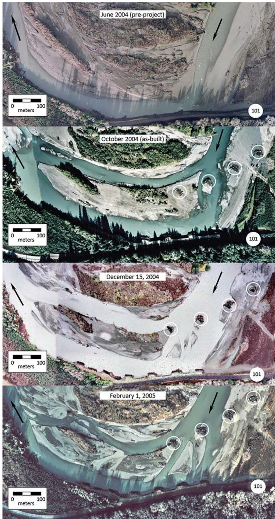
**Fig. 2** Time sequence photos of pre-and post-project conditions for ELJs re-directing flows on the Hoh River, Jefferson County, WA.
