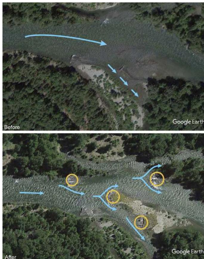
Fig. 11 Four ELJs directing flows into a side channel on the Cle Elum River, before and after conditions.
