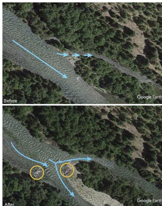
**Fig. 10** Two ELJs directing flows into the upper side channel on the Cle Elum River, before and after conditions. Kittitas County, WA.
