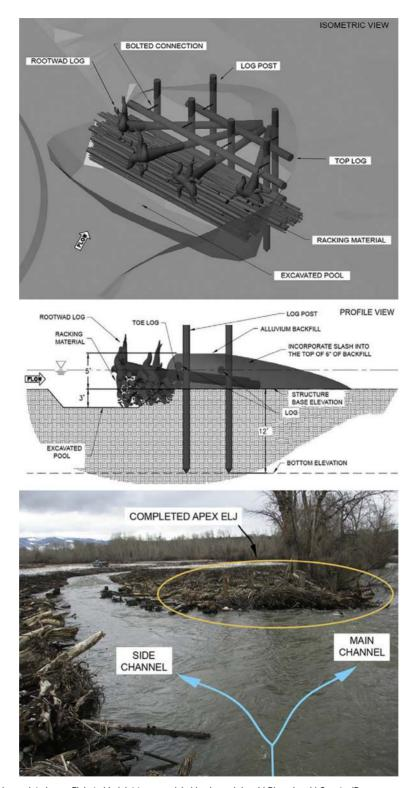
Fig. 20 Design layout and completed apex ELJ at side inlet to perennial side channel, Lemhi River, Lemhi County, ID.
