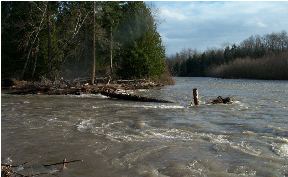
Figure 39. Elwha engineered logjam #99-5 splitting flow between Hunt Road Channel (HRC) and East mainstem channel (EMC), winter 2000. Photo is looking Northeast down EMC.
