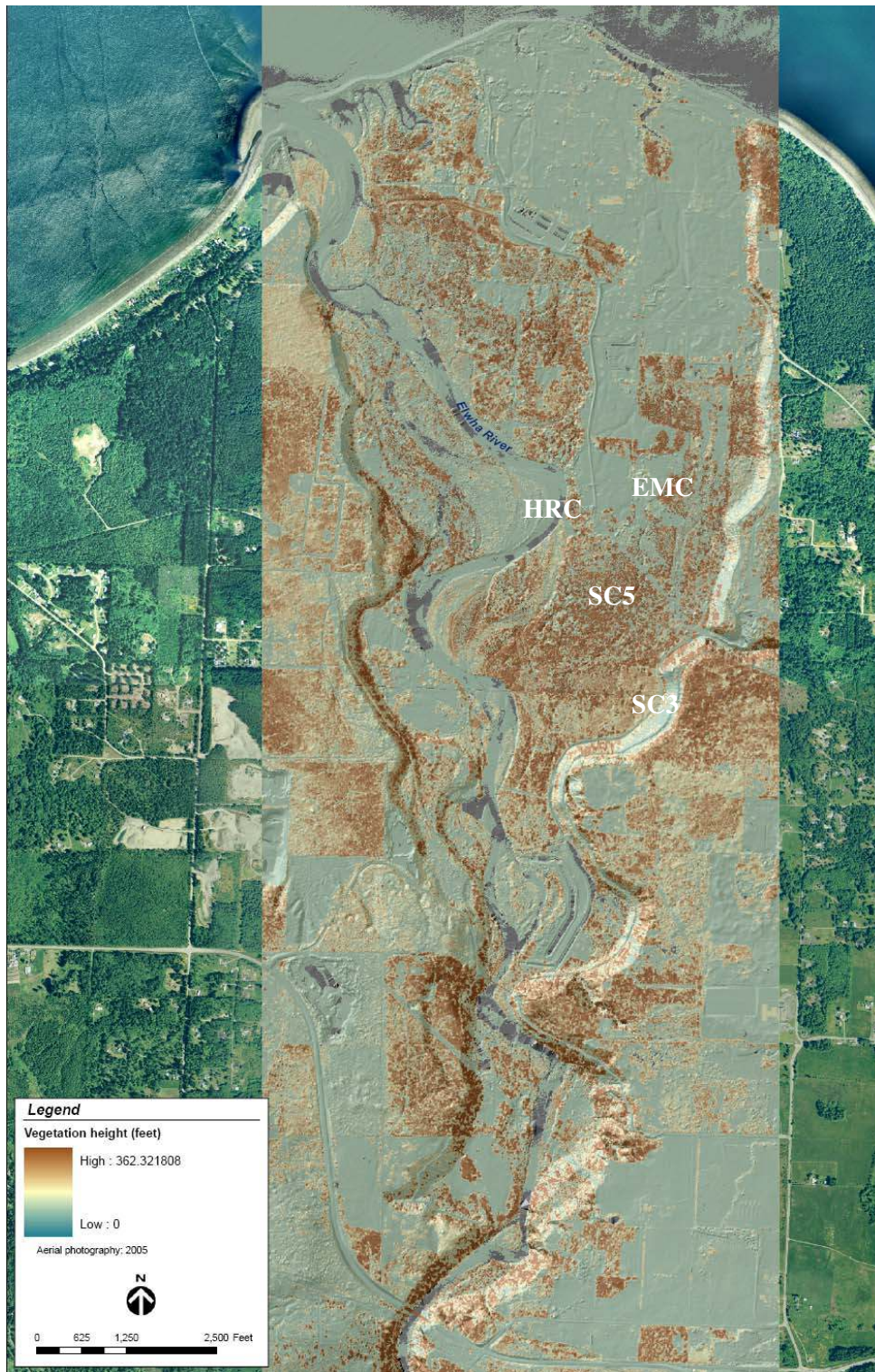
Figure 24. . Height of riparian trees based on differencing of first return and bare earth LiDAR (2004). Note the presence of large trees along the HRC and East of SC3 and SC5.
