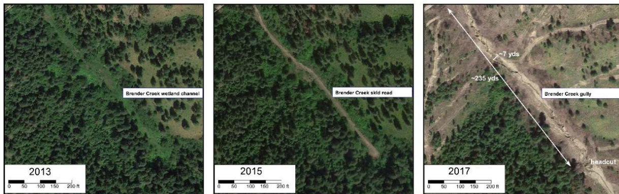
Figure 1a: Example of timber harvest disturbance to second order subsurface alluvial channel, Brender Creek south of the Wenatchee River, Chelan County. Timber skid road was routed up a second order alluvial valley with subsurface runoff (no open water channel). Shortly after logging, a gully formed and evacuate more than 25,000 m 3 of alluvium, converting the channel from subsurface to overland flow.
