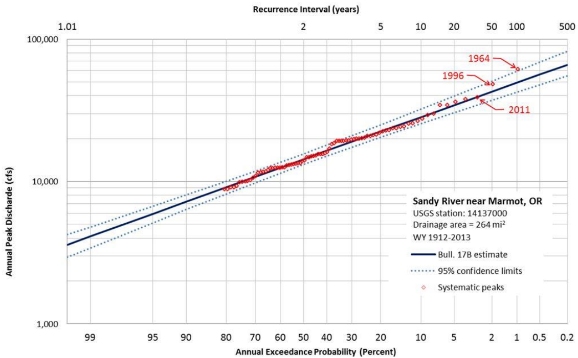
Figure 7B. Flood frequency plot for Sandy River. To determine a flood of a particular recurrence year interval, T, take the reciprocal of the annual exceedance probability (AEP). For example if AEP = 0.01 (1%), then T = 1/.01 = 100 , so an AEP of 1% corresponds to a 100 year flood (1964 flood). An AEP of 2 (1996 flood) corresponds to a 50 year flood. The 2011 flood was about a 30 year flood.
